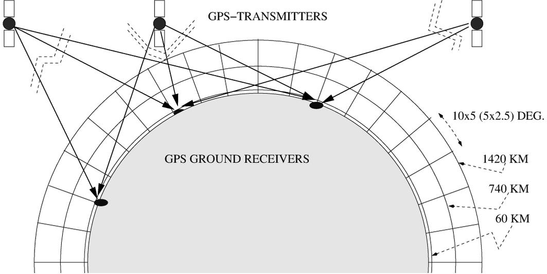
**Figure 1.** Simplified layout of the dual-layer voxel-based tomographic of the ionospheric electron content model, directly estimated from the actual dual-frequency GNSS carrier phase measurements only, by applying a Kalman filter.
