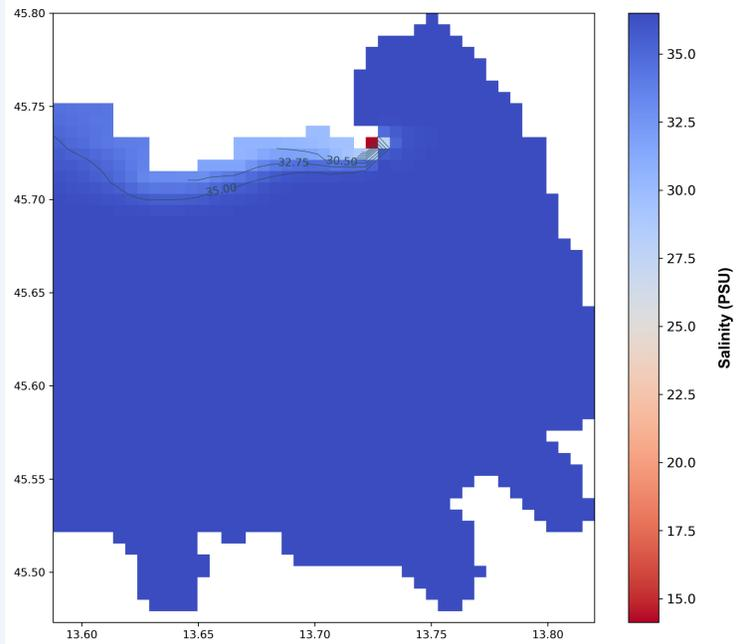
The simulation for the *winter season* was run with initially homogeneous water and a constant bora wind blowing along the Gulf's axis with a speed of  $U = 13$  m/s. The wind stress  $\tau = 0.412$  N/m<sup>2</sup> was obtained with  $\tau = \rho_A C_D U^2$ , where  $C_D = 0.002$  and  $\rho_A = 1.22$  kg/m<sup>3</sup>.
