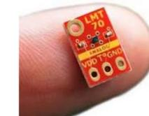
Less than 1mm in diameter, the LMT70 is the world's smallest IC temperature sensor.
