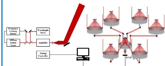
Figure 1 The Schematic diagram of Helium Lidar System
