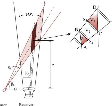
Figure 2 The geometry of the laser beam and the telescope. The darkest shade corresponds to one pixel of the ICCD.
