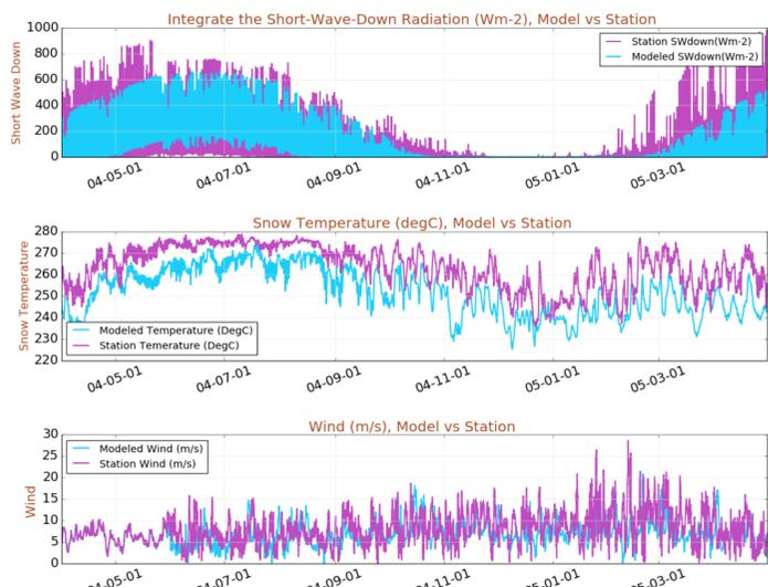
Figure 2: Shows the Data Comparisons of Short-Wave-Down Radiation, Snow Temperature, and Wind Speed from the MAR-Model and Summit-Station in Greenland, from April 1, 2004 to April 30, 2005
