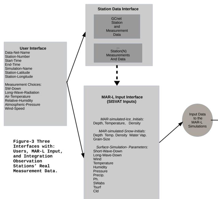
Figure-3 Three Interfaces with: Users, MAR-L Input, and Integration of Observation Stations' Real Measurement Data.
