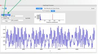
Data Processor -> SSA – de-compose data or target on empirical orthogonal components and reconstruct a signal with selected components using Singular Spectrum Analysis.
