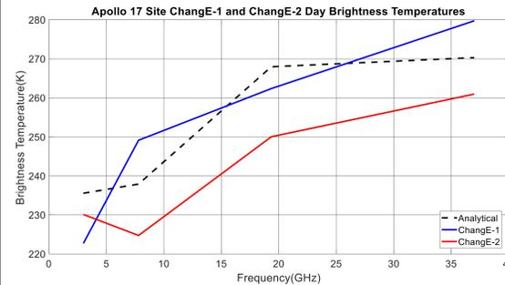
**Figure 3.** Average surface brightness temperatures measured by Chang'E-1 and Chang'E-2 over the Apollo 17 site during lunar days compared with the analytical calculations. Although the trends are similar, the differences between measured and simulated brightness temperatures can be as large as 20 K.
