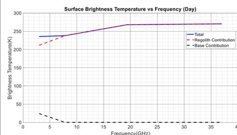
**Figure 7.** Surface brightness temperatures at Chang'E-1 and Chang'E-2 frequencies for a 5-meter regolith with rock base. Notice that brightness temperatures at low frequencies may be sensitive to the bedrock.
