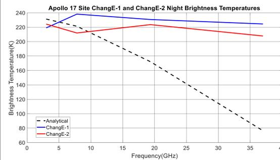
**Figure 4.** Average surface brightness temperatures measured by Chang'E-1 and Chang'E-2 over the Apollo 17 site during lunar nights compared with the analytical calculations. Simulated brightness temperatures are found to be much lower than the actual measurements at high frequencies which requires further investigations.
