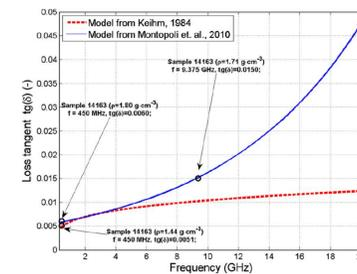
**Figure 5.** Electromagnetic loss tangent models for lunar regolith [4].
