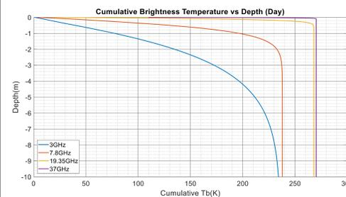
**Figure 6.** Cumulative brightness temperatures found by summing emissions from the surface to each depth at Chang'E-1 and Chang'E-2 frequencies. Notice that as frequency increases contributions from the deeper layers decreases. Higher frequencies are sensitive to only very shallow regolith.
