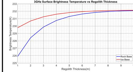
**Figure 8.** 3 GHz surface brightness temperatures computed for regolith on rock and ice bases versus the regolith thickness. Notice the significant impact of the bedrock type on surface brightness temperatures for thinner regolith.
