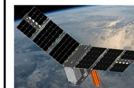
**Figure 10.** Recent developments in radiometer design and CubeSat technologies may enable future lunar missions which carry wideband microwave radiometers for passive remote sensing of lunar regolith and bedrock. The figure demonstrates the CubeRRR (CubeSat Radiometer RFI Technology Validation) instrument which carries a microwave radiometer operating in the 6-40 GHz band [7].
