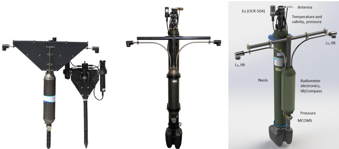
Figure 1: Left to right: The freefall (without Navis float) HyperNAV configuration shown next to a Sea-Bird Scientific HyperPro II series; HyperNAV configuration (mounted on a Sea-Bird Scientific Navis float); Rendering of the HyperNav system showing associated instrument locations.
